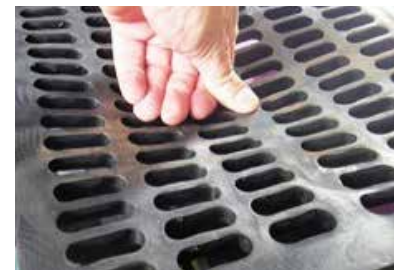
Under 20kg load, a 50mm deflection
