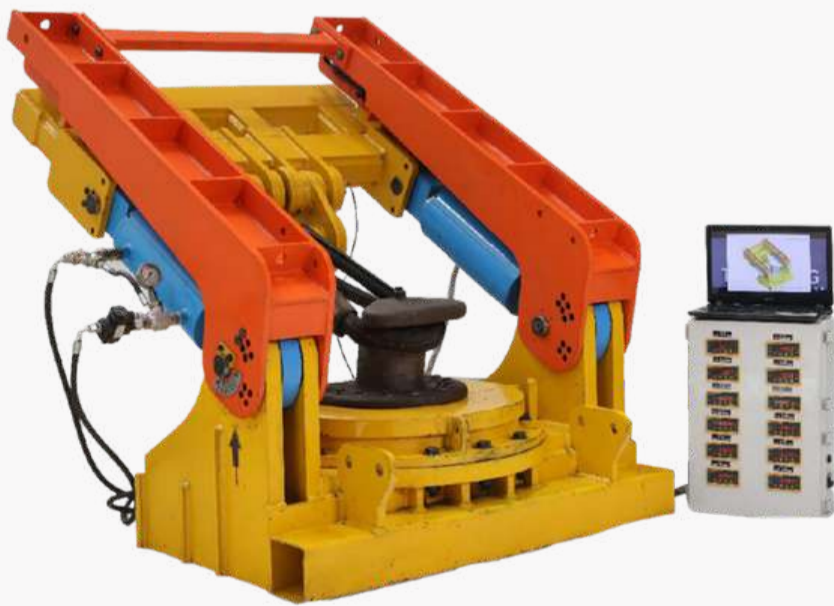
TRELLEBORG BOLLARD TESTING MACHINE
