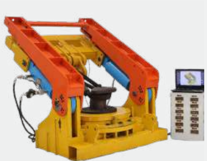
BOLLARD TESTING MACHINE
