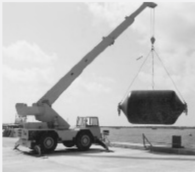
Fender with chains oriented incorrectly. Note damage to the fender ends.
