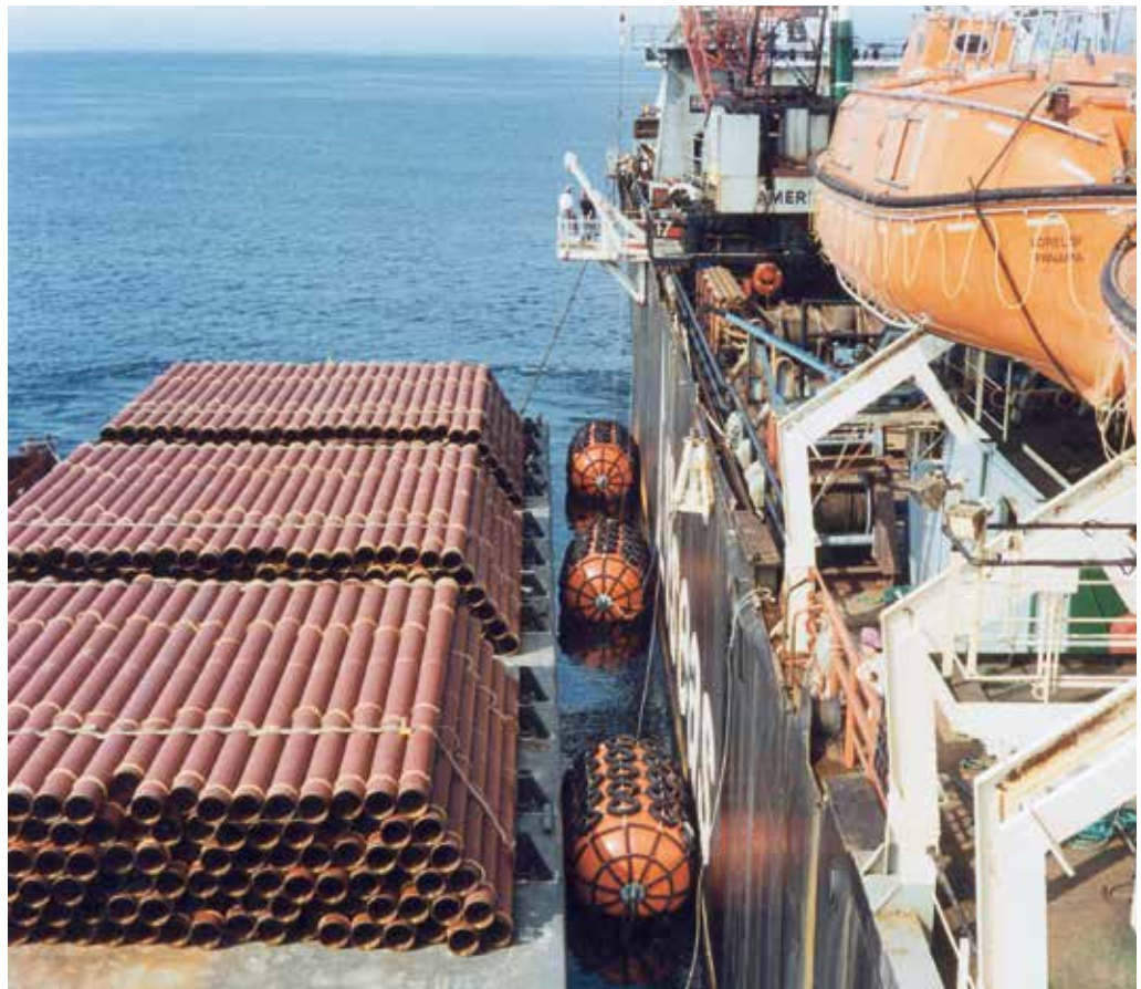
Trelleborg Marine Systems Foam Fenders protecting Allseas BV 'Lorelay' pipelay vessel.
