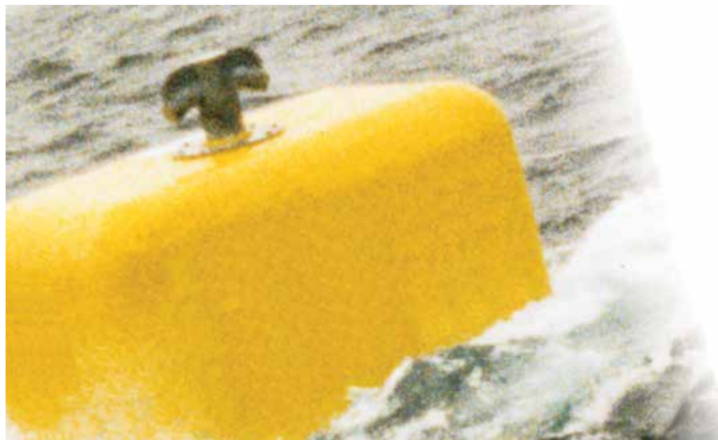
An 18,000 kg suitcase type Anchor Pendant Buoy on station in the North Sea.
