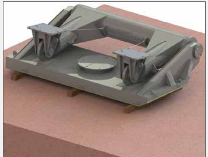
Figure 4: PMF unit placed on timber/ rubber blocks
