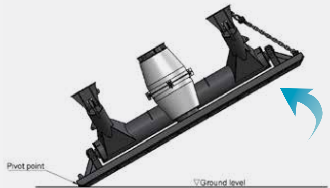
Figure 10: PMF unit assembly lifting
