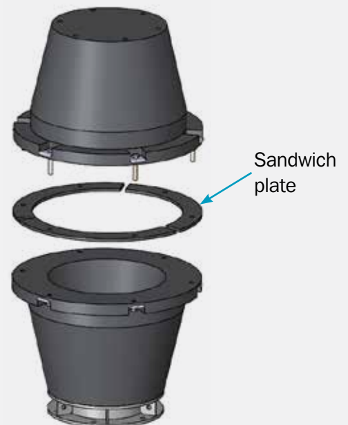
Figure 6: Assembling "back-to-back" SCN fenders
