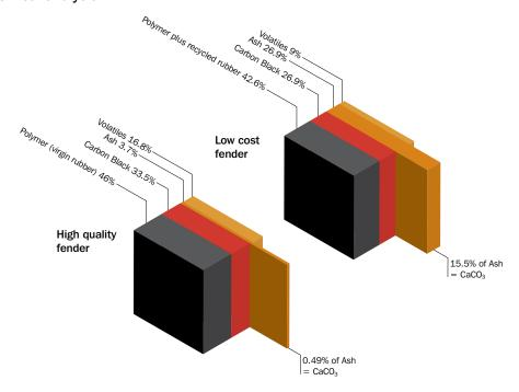
$NB: Carbon \ Black \ is \ the \ high \ quality, \ reinforcing \ filler. \ Ash \ contains \ CaCO_3, \ the \ non-reinforcing \ white \ filler.$
