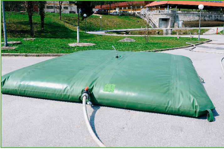
Fig. 5.12: Filling of the tank
