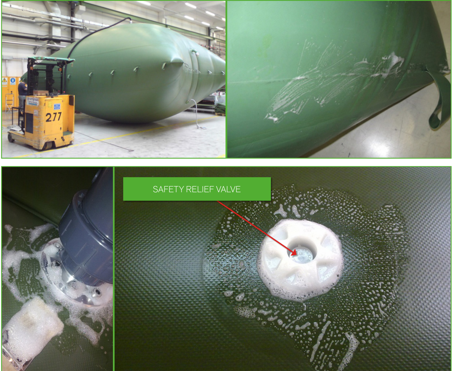
Fig. 8.10: Test of the repaired closed tank
