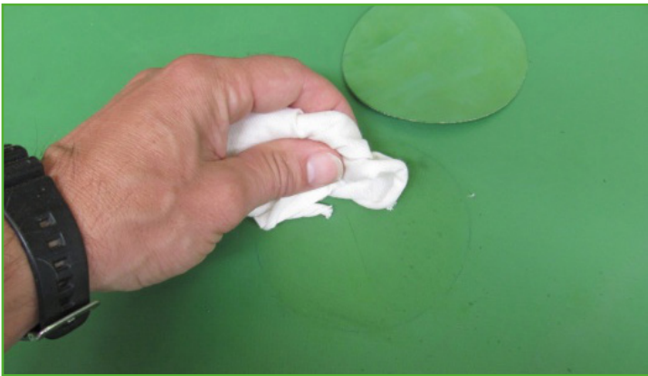
Fig. 8.5: Clean the glued area
