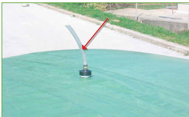
Fig. 5.8: Threaded air vent with a hose
