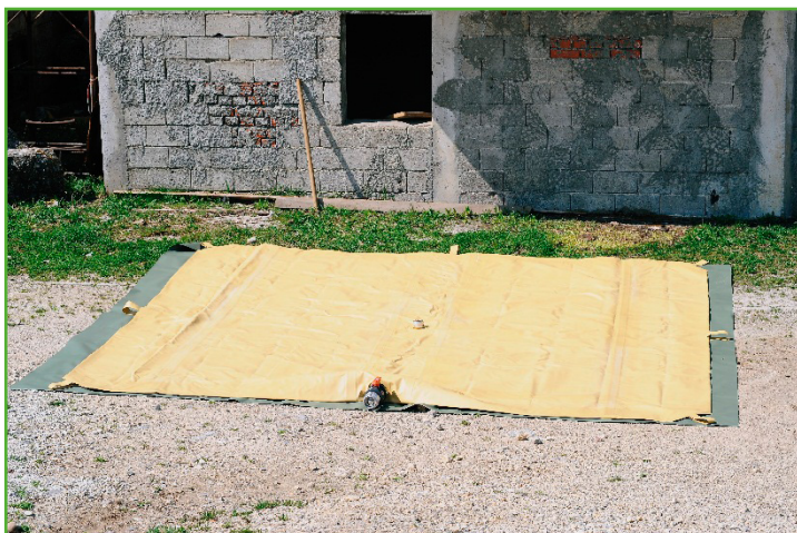
Fig. 5.7: Straighten up the closed rubber tank over the surface
