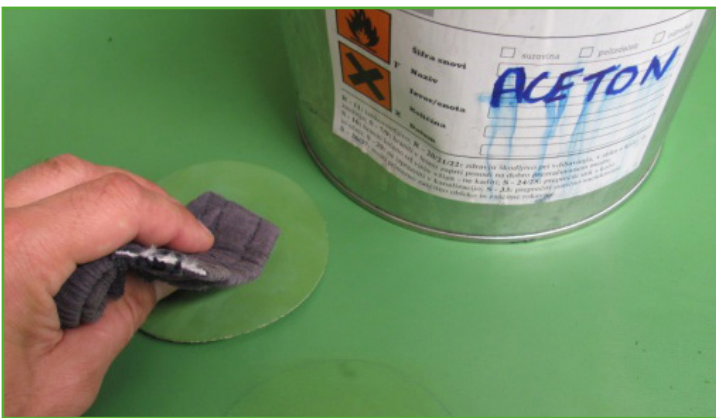
Fig. 8.6: Clean the area to be glued with acetone
