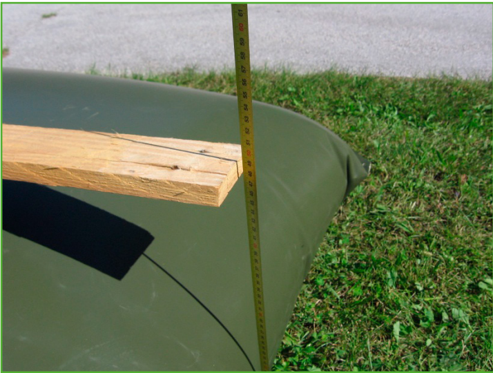
Fig. 5.13: Measure the filled tank from the ground to the lath's edge using a tape measure
