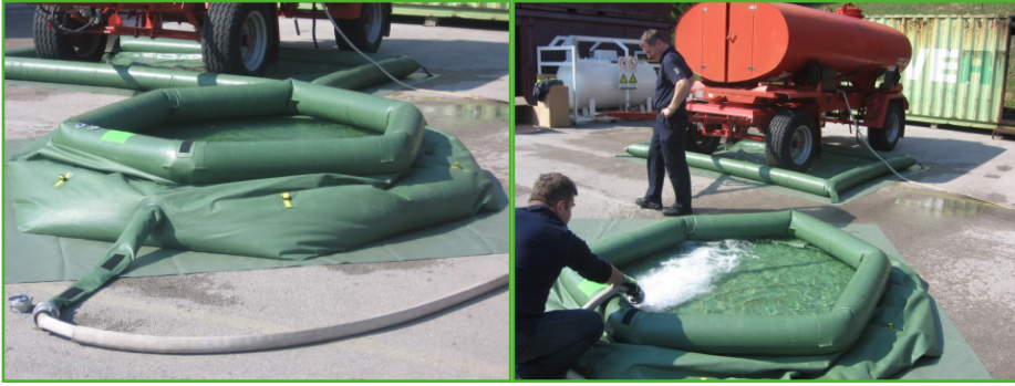
Fig. 8.11: Test of the repaired open tank
