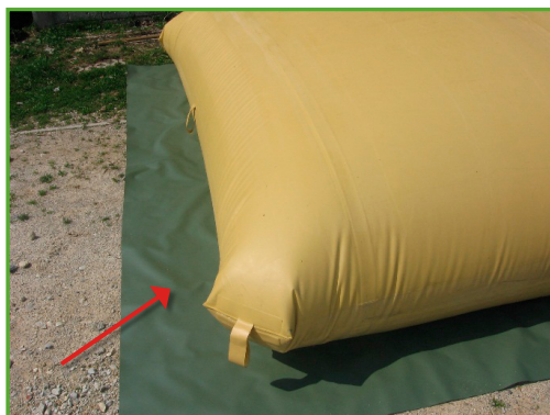
Fig. 5.5: Protective pad under the rubber tank
