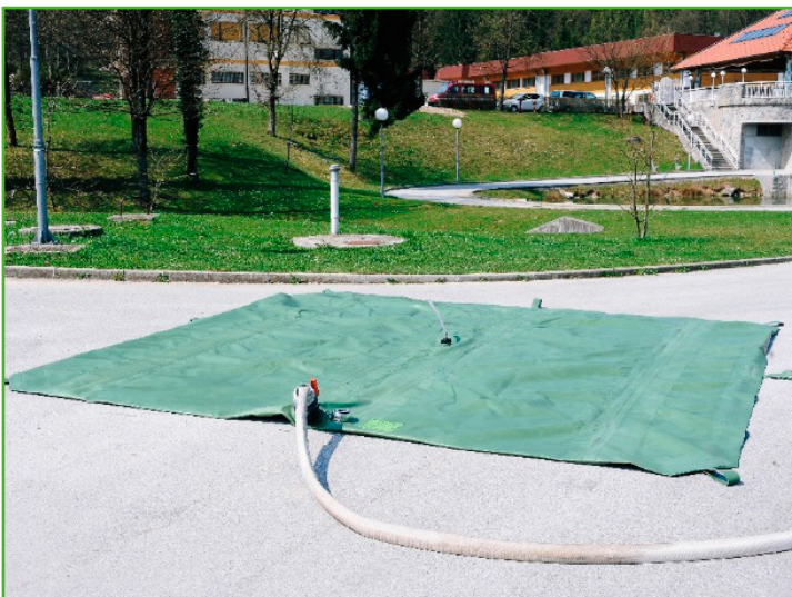
Fig. 5.11: Tank with the connected supply hose
