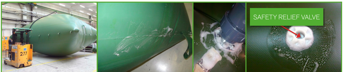
Fig. 5.2: Air tightness test with soapy water
