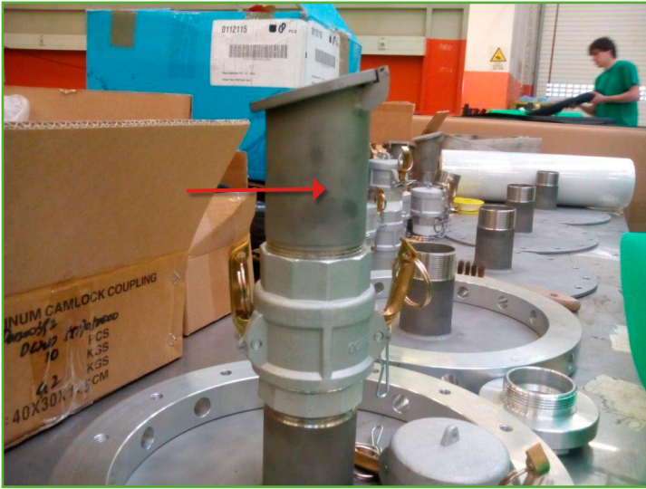
Fig. 5.9: Air vent with a cap mounted on a camlock coupling
