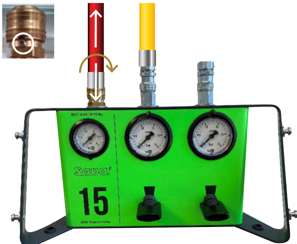
Figure 7.14: Disconnecting the inflation hose from the controller.
