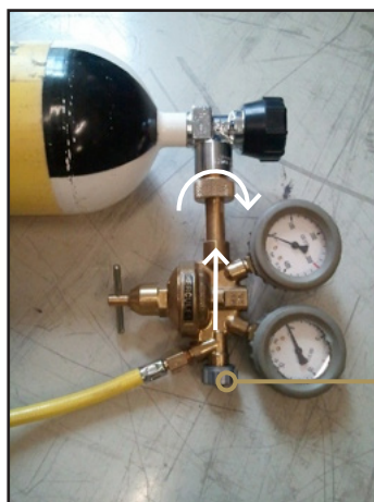
Figure 7.10: Installing the pressure reducing valve.
