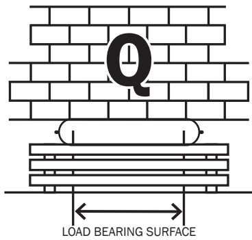
Figure 7.18: Reducing the load-bearing surface with increasing the lifting height.
