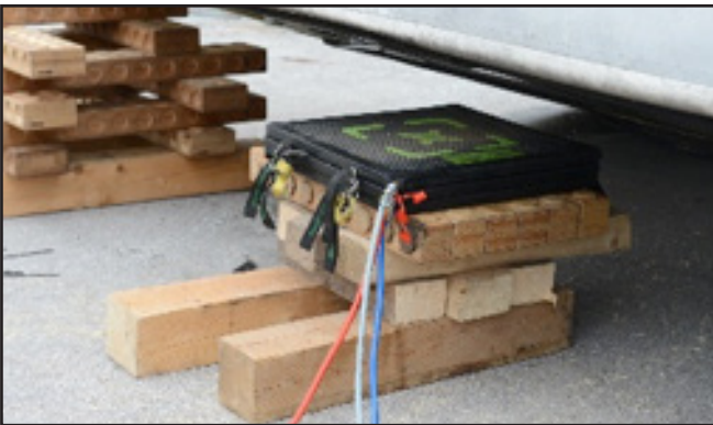
Figure 7.6: Positioning SAVA lifting bag on a lifting site.
