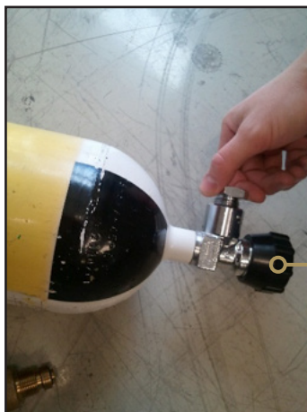
Figure 7.9: Removing the safety plug from the pressure vessel.
