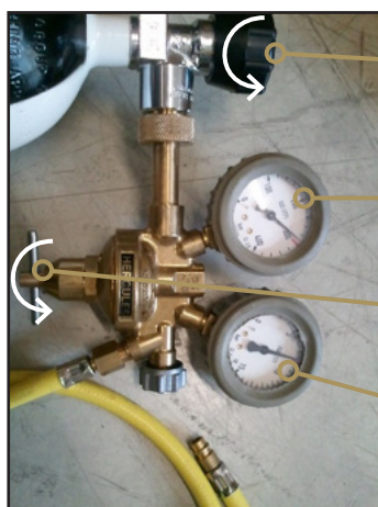
Figure 7.11: Setting the pressure reducing valve.
