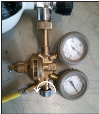
Figure 7.13: Releasing the relief valve.
