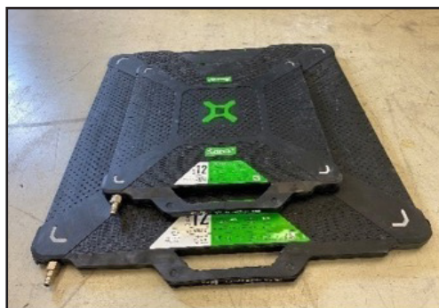
Figure 7.24: Combining conventional SAVA lifting bags to increase the lifting height.
