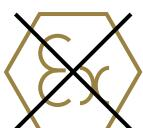
The standard version of Sava lifting bags is NOT intended for use in potentially explosive atmospheres.
