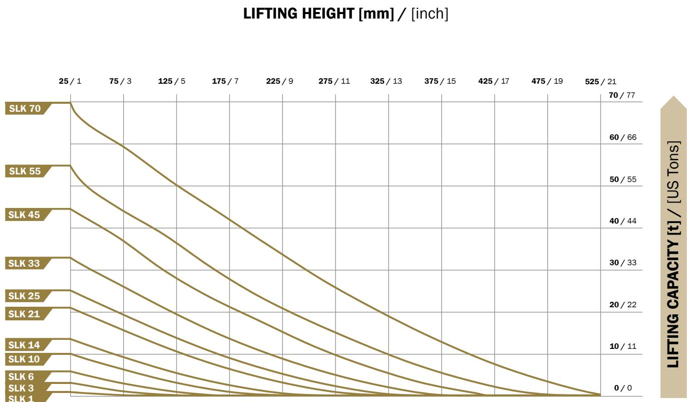
**Graph 6: Lifting capacity of high-pressure lifting bags SLK-L**
