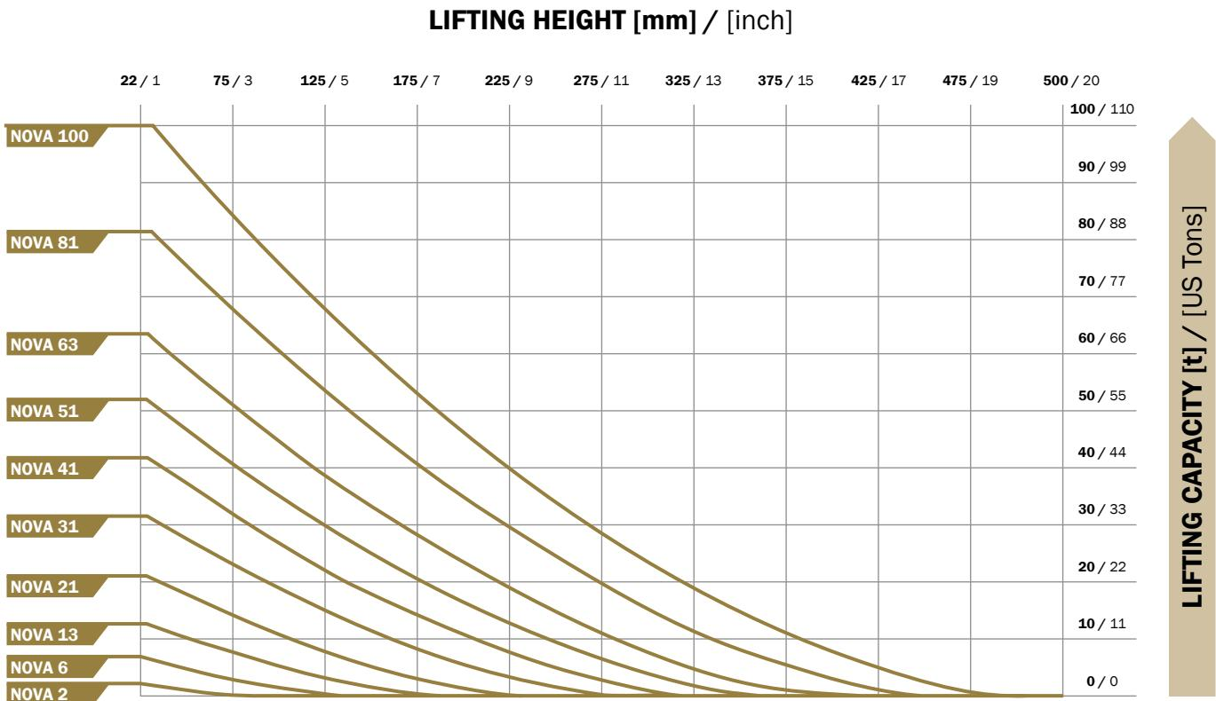
**Graph 2: Lifting capacity of high-pressure lifting bags NOVA 2, NOVA 6, NOVA 13 in NOVA 21**
