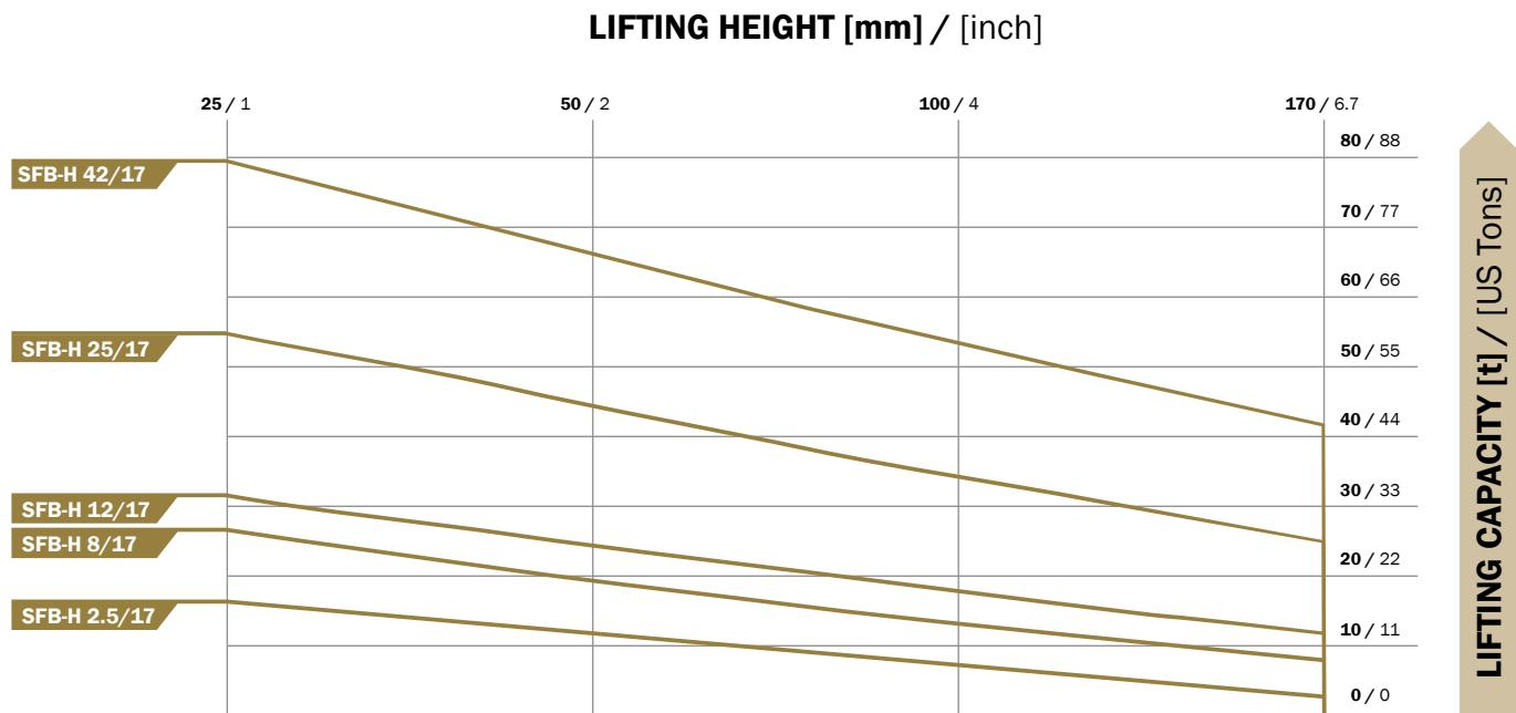
**Graph 10: Lifting capacity of high-pressure lifting bags VEGA Flat**
