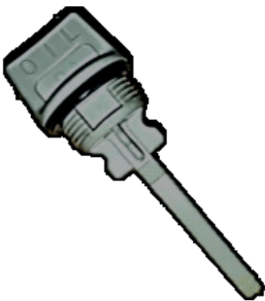
Fig. 2: Oil dipstick for oil level check
