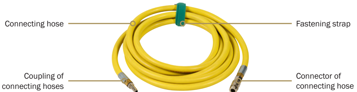
Figure 7.3: Connecting hose – schematic presentation.
