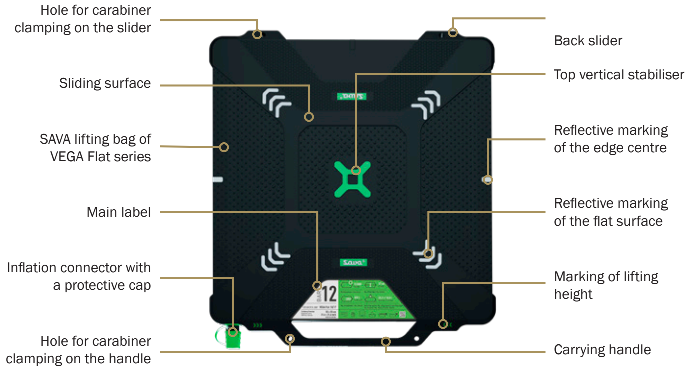
Figure 6.1: Schematic description of SAVA lifting bag
