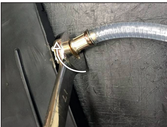
Figure 40: Screwing the new coupling
