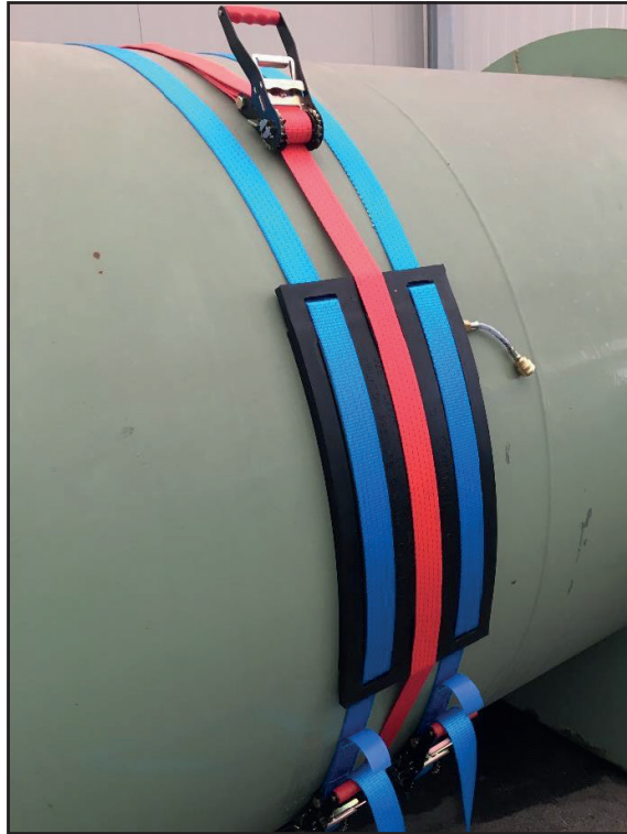
Figure 9: The fastened SAVA sealing bag M 1/6 or M 1/10 with three straps
