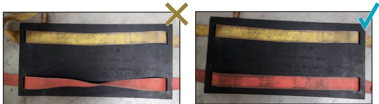
Figure 6: Incorrectly fed orange strap (left) and correctly fed strap (right)
