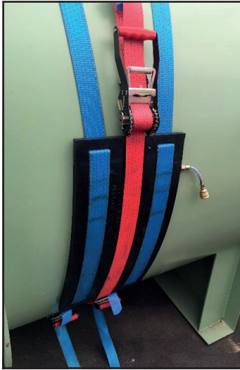
Figure 32: SAVA sealing bag of M 1/6 or M 1/10 type with all three ratchet straps attached
