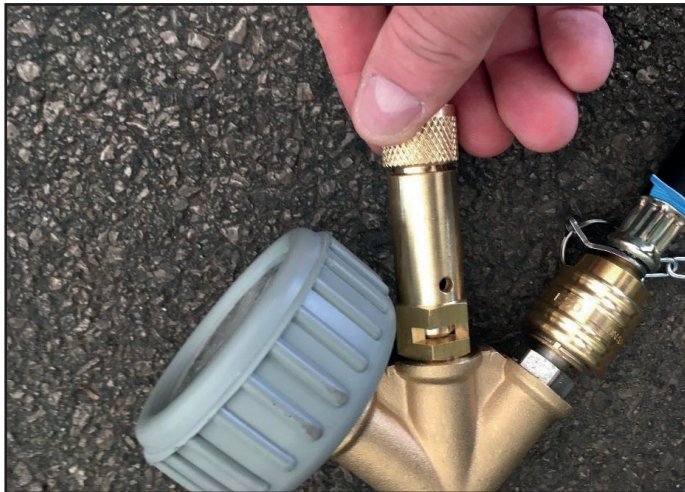
Figure 17: Opening the safety valve screw
