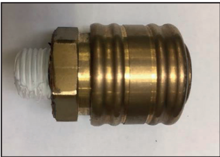
Figure 22: The thread wrapped with teflon tape
