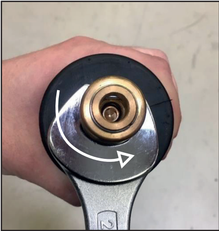
Figure 21: Unscrewing the coupling
