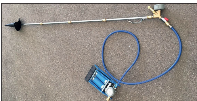
Figure 18: SAVA sealing cone prepared for use
