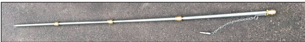
Figure 5: Four inflation rods connected together
