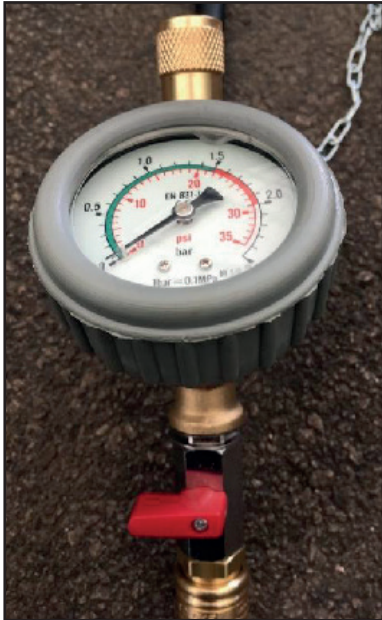
Figure 15: Valve on the controller in closed position
