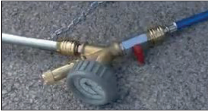
Figure 9: Inflation hose connected to the controller
