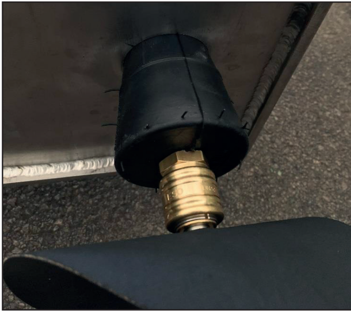
Figure 19: SAVA sealing cone inserted in the damaged surface
