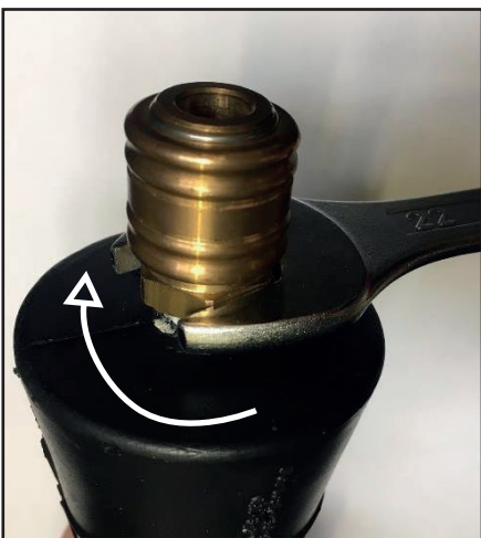
Figure 23: Screwing the new coupling
