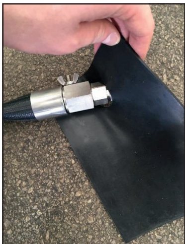
Figure 11: Mounting the sealing plate on the SAVA sealing hose
