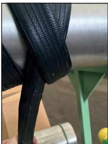
Figure 13: A knot on one end of the SAVA sealing tube
