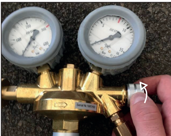
Figure 4: Closing the relief valve (left) and the gasket in the inflation connector (right)
