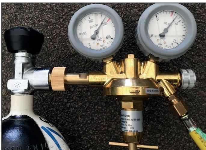
Figure 6: Pressure in the pressure vessel (left pressure gauge) and set reduced pressure (right pressure gauge)
