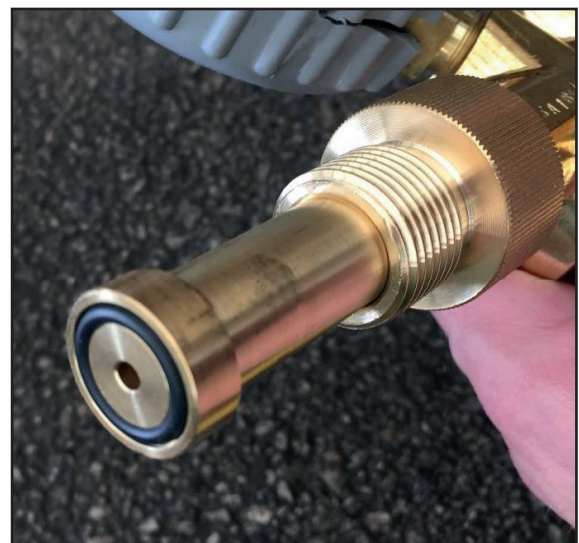
Figure 4: Closing the relief valve (left) and the gasket in the inflation connector (right)
