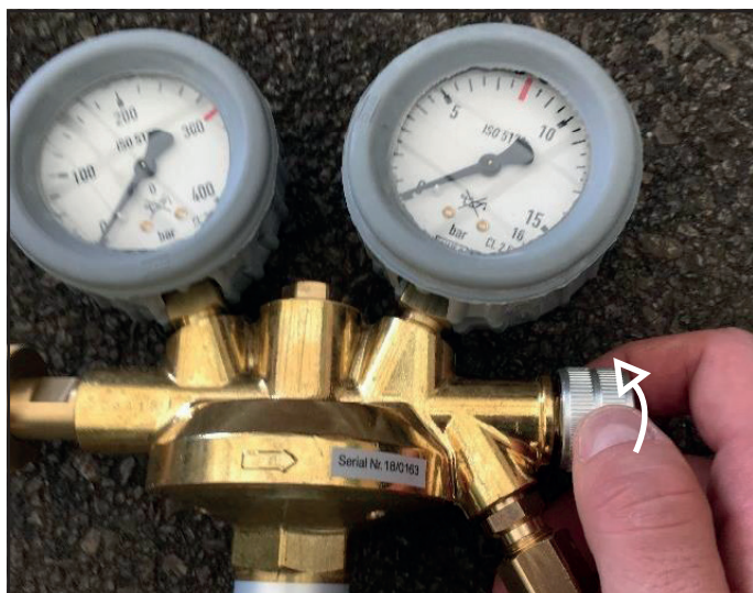
Figure 19: Opening the relief valve on the pressure reducer
