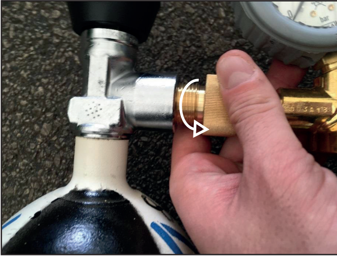
Figure 9: Unmounting the pressure reducer from the pressure vessel
