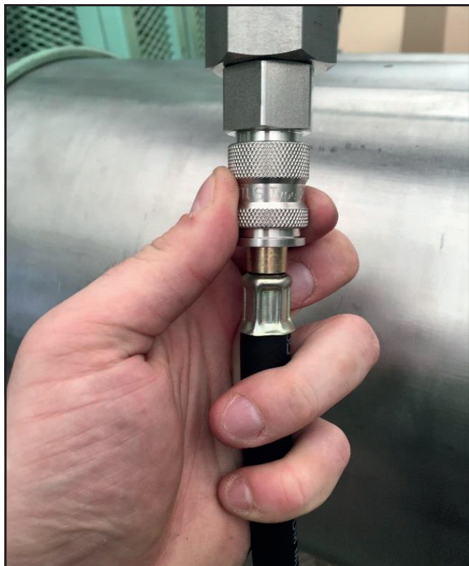
Figure 23: Uncoupling of the inflation hose from the SAVA sealing hose
