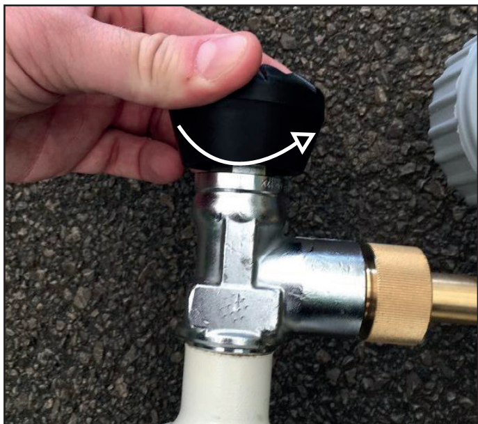
Figure 8: Closing the valve on the pressure vessel
