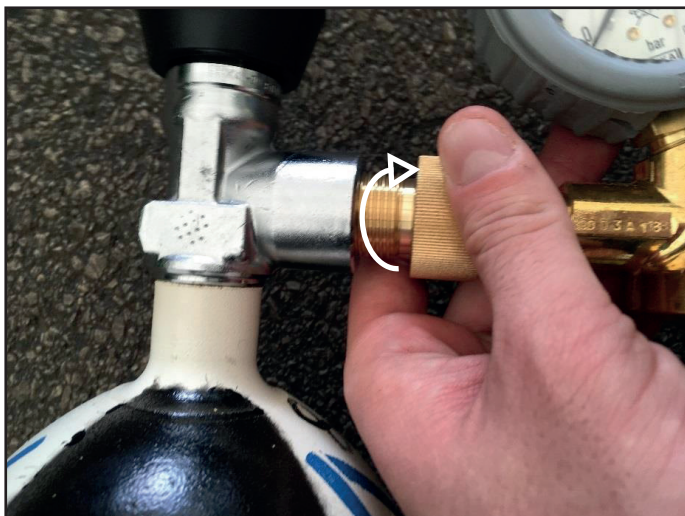
Figure 5: Mounting the pressure reducer on the pressure vessel
