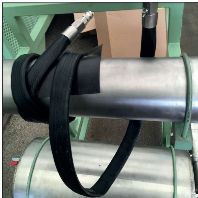
Figure 24: Removing the SAVA sealing hose
