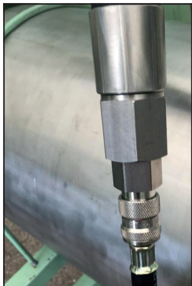
Figure 17: Inflation hose connected to the SAVA sealing tube
