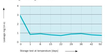
FlatSeal<sup>TM</sup> HMF66 offers effective sealing performance after initial temperature exposure in the application. Tightness tests at room temperature without previous temperature increase are not indicative of actual performance.
