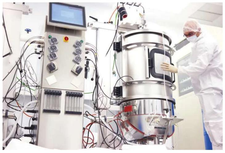
Biopharmaceutical companies utilize a single-use system to manufacture vaccines using large scale bioreactor bags.
